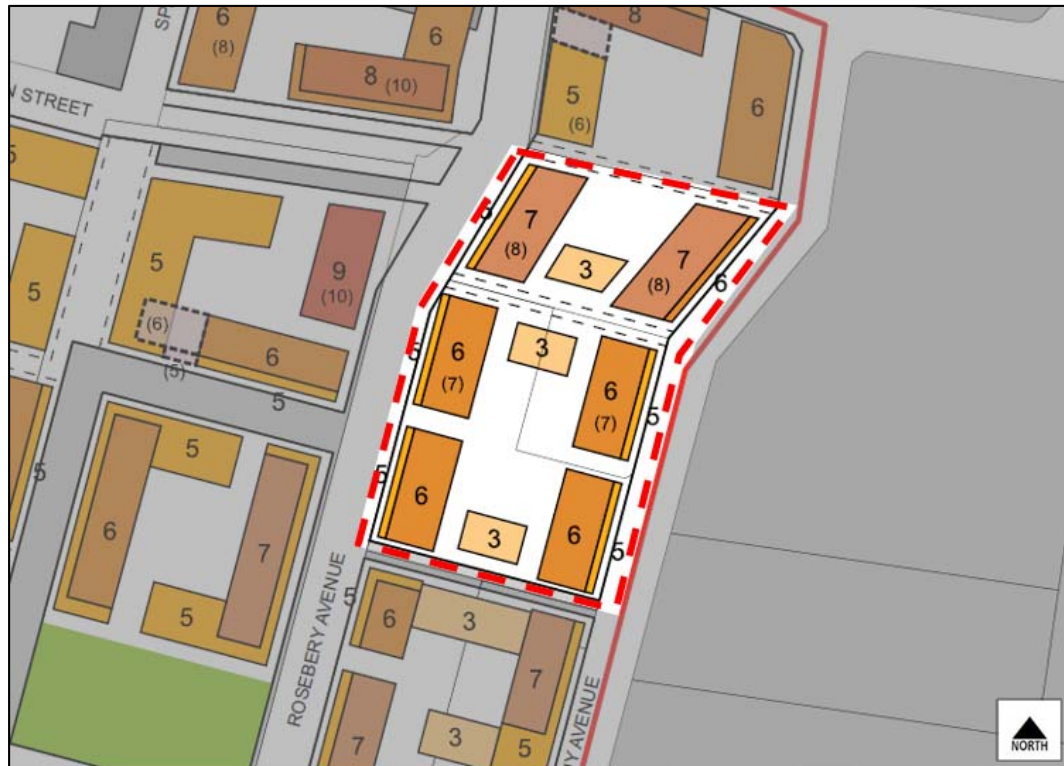
Figure 4: Block plan of the proposed scheme. Height in storeys indicated for each building.
